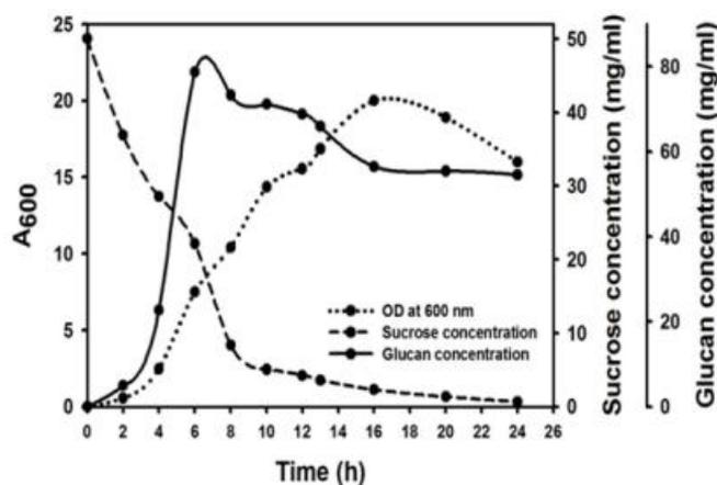
**Figure 4.** Validation of data for glucan production in bioreactor. Variation of glucan concentration (mg/ml), sucrose concentration (mg/ml) and cell optical density ( $A_{600}$ ) during batch fermentation of *Pediococcus pentosaceus* CRAG3 in bioreactor.
