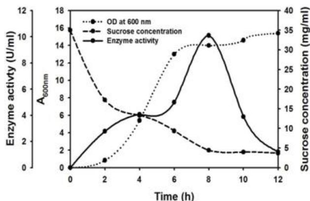
**Figure 2.** Validation of data for glucansucrase production in bioreactor. Variation of glucansucrase activity (U/ml), sucrose concentration (mg/ml) and cell optical density ( $A_{600}$ ) during batch fermentation of *Pediococcus pentosaceus* CRAG3 in bioreactor.**Table 7.** Response table of means for glucan production by *Pediococcus pentosaceus* CRAG3.
