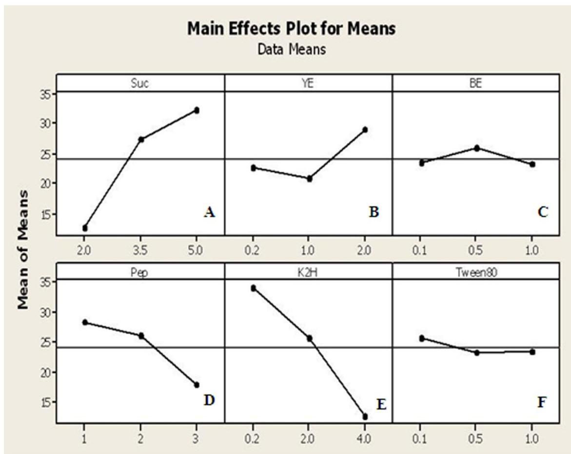
**Figure 3.** Impact of selected fermentation factors and their assigned level on glucan production by *Pediococcus pentosaceus* CRAG3. X-axis represents assigned levels of selected factor (% w/w or w/v) and Y-axis represents glucansucrase production (U/ml). (a) Sucrose, (b) Yeast extract, (c) Beef extract, (d) Peptone (e)  $K_2HPO_4$  and (f) Tween-80.
