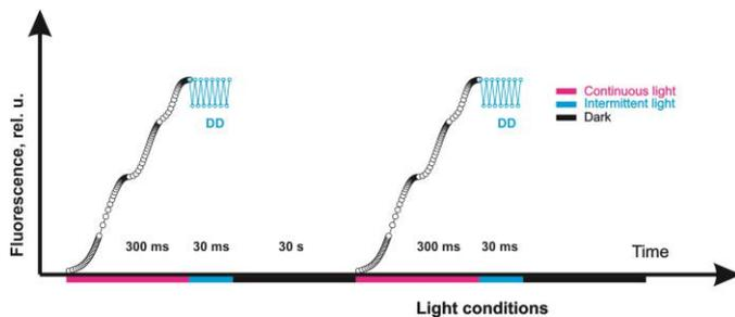
**Figure 5.** Schematic representation of the structure of Protocol 4. Two measurements – one of 300 ms and the other of 30 ms with saturating light of  $4000 \mu\text{mol photons}\cdot\text{m}^{-2}\cdot\text{s}^{-1}$  are repeated 21 times. Between every measurement a dark interval of no illumination or illumination with 50, 100, 150 or  $200 \mu\text{mol photons}\cdot\text{m}^{-2}\cdot\text{s}^{-1}$  is applied.
