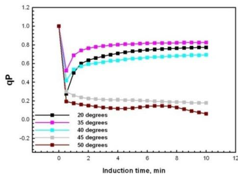
**Figure 12.** Changes in the dynamics of  $qP$ , measured with Protocol 4 in samples, treated with different temperatures (20, 35, 40, 45 and 50°C) during the measurement.
