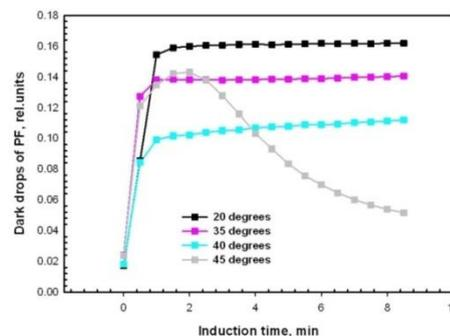
**Figure 8.** Changes in the DD of PF, measured with Protocol 3 in samples, treated with different temperatures (20, 35, 40 and 45°C) during the measurement. The intervals between the light pulses are with no background illumination.
