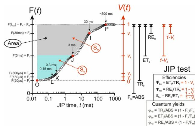
**Figure 1.** Induction Curve of the PF signal, measured with MPEA. The OJIP characteristic points are presented. Some of the parameters that can be directly derived are shown.
