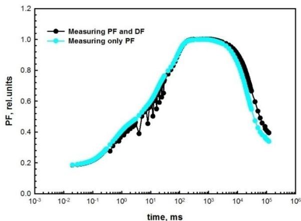
**Figure 3.** Induction curves of PF, measured with Protocol 1 (see Materials and methods). The duration of the record is 120 sec. Illumination is saturating –  $4000 \mu\text{mol photons}\cdot\text{m}^{-2}\cdot\text{s}^{-1}$ . Blue curve presents the form of the curve without application of Dark intervals. Black curve shows the DD dips, formed when the light is switched off for measuring of DF.
